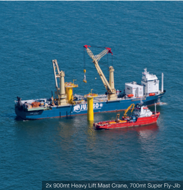
2x 900mt Heavy Lift Mast Crane, 700mt Super Fly-Jib
